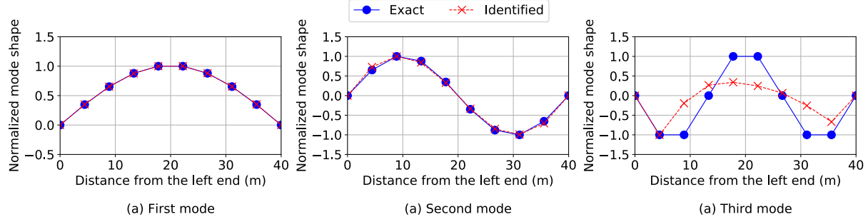
Figure 21 - The first three normalized mode shapes identified from matrix D obtained by Lagrange mapping
