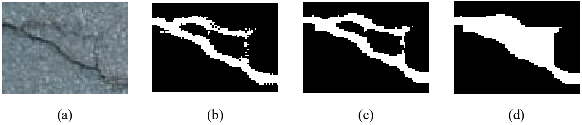
Fig. 6. Issues with deconvolution layer output (a) original patch; (b) raw output; (c) after 3×3 morphological operations; (d) after 15×15 morphological operations
